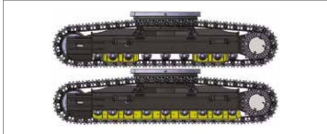
**Track guards:** to provide better protection, track alignment, and performance of machine while travelling, 3 guards per track as standard or DX490LC-7K & DX530LC-7K (full-length track guard optional) and, for DX420LC-7K, 2 guards per track as standard (double and full-length track guards available as options). These various track guard options provide you with optimal solutions for your extreme applications.
