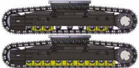
**Track guards:** to provide better protection, track alignment, and performance of machine while travelling. 2 guards per track as standard (double and full-length track guards available as options). These various track guard options provide you with optimal solutions for your extreme applications.
